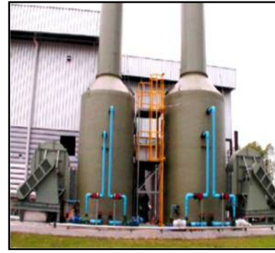
EMR 型喷淋洗涤塔 Spray tower TYPE EMR
