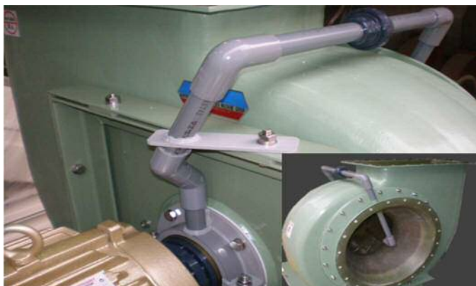
环绕式轴封 GLAND BYPASS TYPE (FAN)
